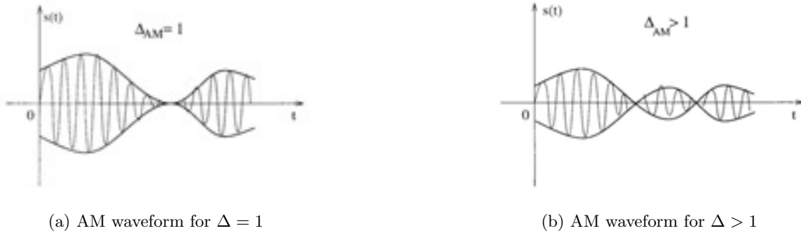
Figure 2.6: AM waveforms for various \Delta values
